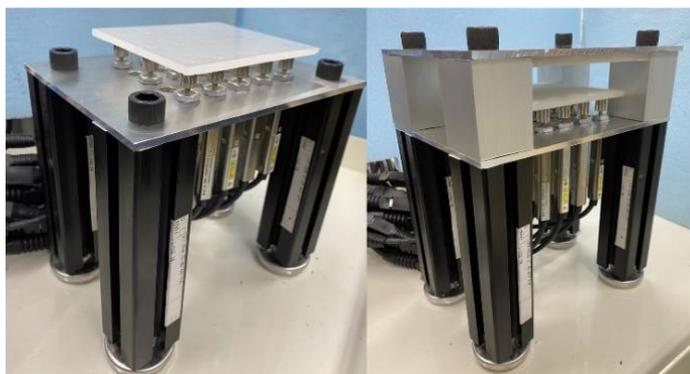
Fig. 1 Device simulating mastication
